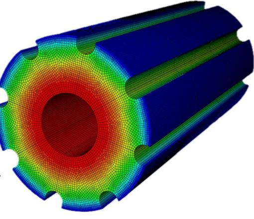
Example of an element-wise temperature distribution that can be imported in MCNP6.4+ via an HDF5 mesh file
