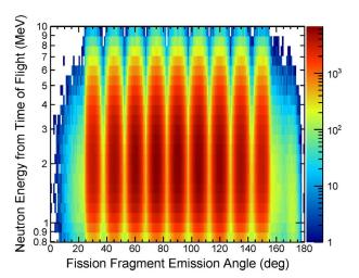
The matrix connecting measured neutron energy from time of flight to fission fragment emission angle in the Chi-Nu experimental environment resulting from connection of CGMF calculations to MCNP6 simulations with PTRAC output. Neutron detectors are placed at 15 deg increments from 30-150 deg, yielding the observed pattern in this spectrum.
