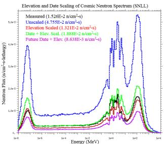
**Fig. 2.** Neutron background spectrum at SNLL location 37° N, 120° W, 196 m with the effects of scaling.
