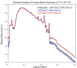
**Fig. 1.** Elevation scaling of the cosmic-photon background near the Albuquerque International Airport.
