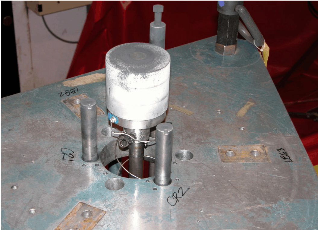
Figure 23. Mounting Plate with Control Rods, Burst Rod, and Safety-Block Subassembly.
