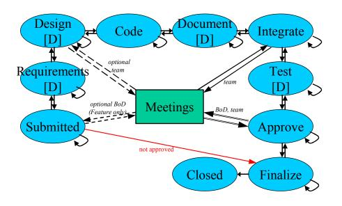
Figure B2. Features, Enhancements, and Bugs Development Subprocess
