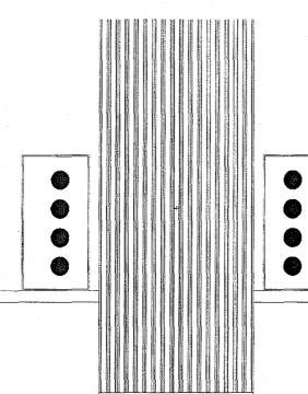
Fig. 3. MCNP model showing a slice through both heads of the detector, each with four <sup>3</sup>He detector tubes, with the 17 x 17 fuel bundle centered between the heads.
